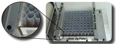
**(c)** Using the Adjustment Screws, position the adjustable Front and Back Guide Plates such that the edges are nearly touching the vials. This will minimize excess film that results in undesirable overhang on sides of vials.
